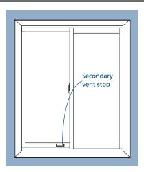
With the wide part of the catch toward the sash, put the catch end in first and then press the other end of the device into the secondary vent stop cavity until it snaps into place. Some adjustments to the hole may be required if it is not large enough for the new device.
