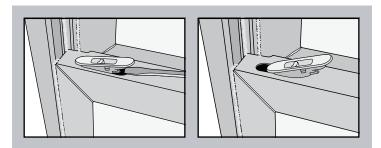
4. At an angle, insert the replacement tilt latch into the hole in the sash.
