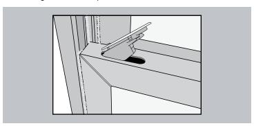
5. When fully inserted, press the tilt latch down until it snaps into place and is flush with the sash.
