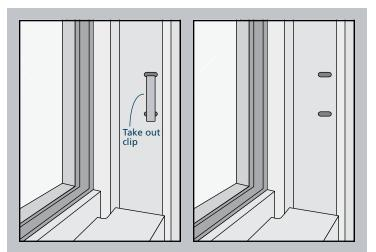
3. Using a flat head screwdriver, pry the top of the clip from the slot until it pops out. Remove the clip from the bottom slot.
