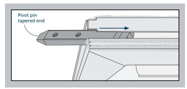
5. Install the screw (do not over tighten and strip the vinyl) in the new pivot pin and reinstall the sash.
