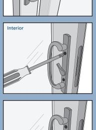
4. Install the blind nuts on the exterior and the screws on the interior.
