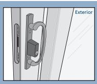
2. Remove the two screws on the interior handle and remove.
