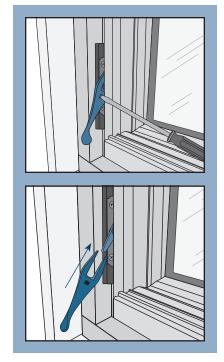
3. Slide the new lever onto the lock until it snaps into place.
