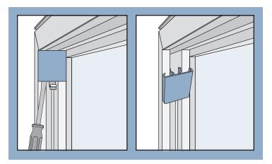
3. If needed lift sash to move the stop into place.
